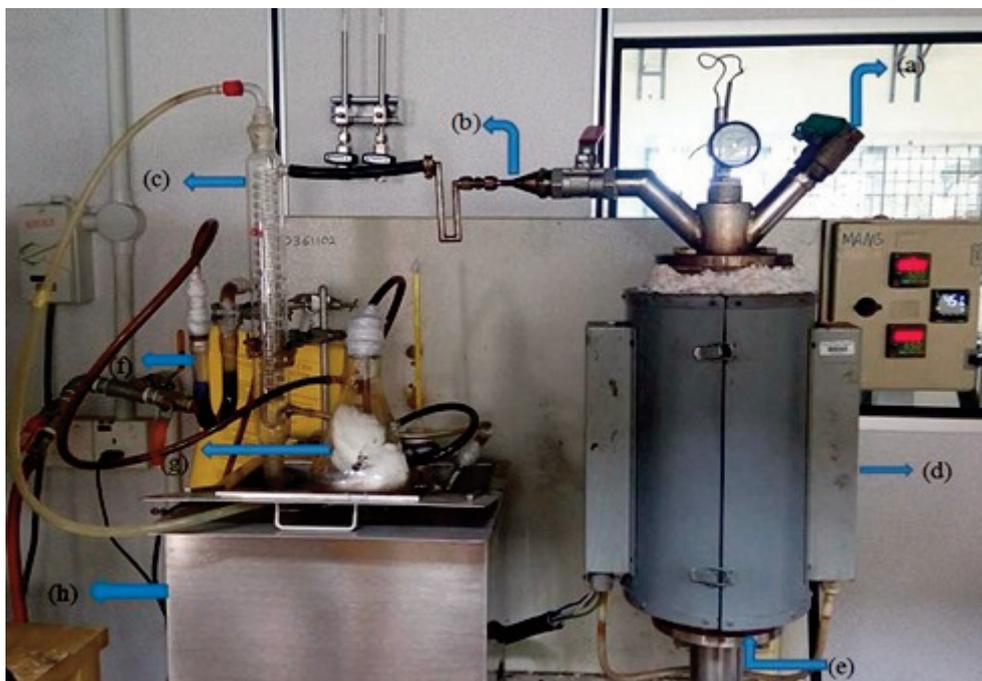
Figure 1. A complete preview of the gasifier reactor and other parts (a) feedstock inlet, (b) syngas outlet, (c) condenser, (d) reactor, (e) air inlet, (f) silica gel, (g) tar collection cotton, (h) ice-water
