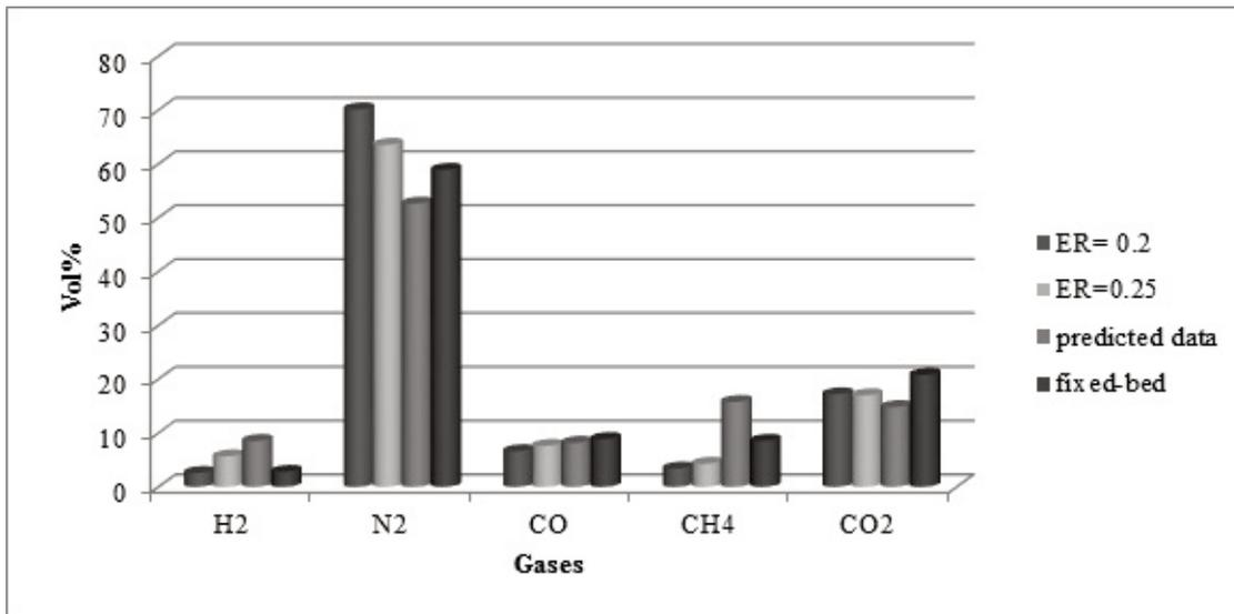
Figure 4. Comparison of experimental data in different modes with predicted data at 750<sup>o</sup>C
