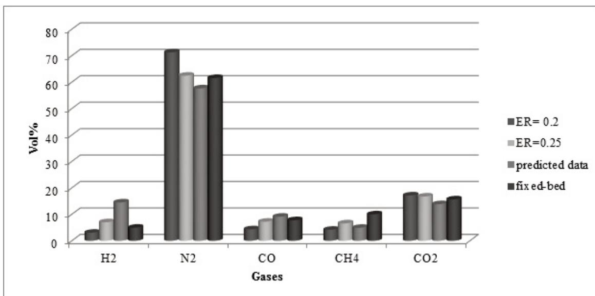
Figure 5. Comparison of experimental data in different modes with predicted data at 800<sup>o</sup>C
