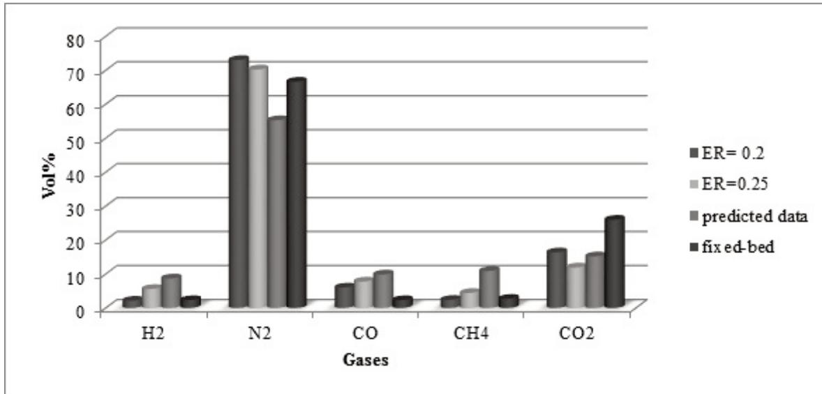
Figure 2. Comparison of experimental data in different modes with predicted data at 650°C
