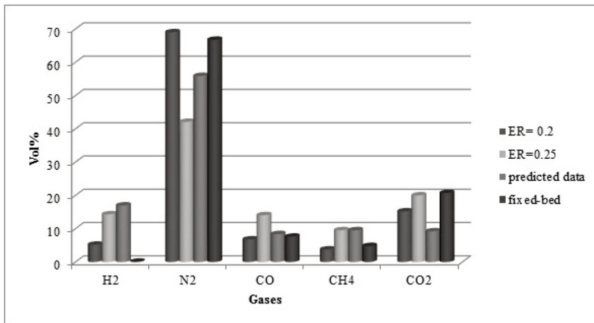
Figure 6. Comparison of experimental data in different modes with predicted data at 850°C
