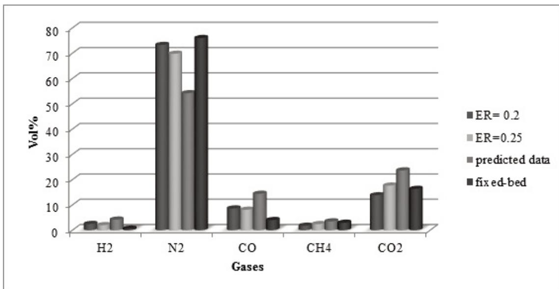
Figure 3. Comparison of experimental data in different modes with predicted data at 700°C
